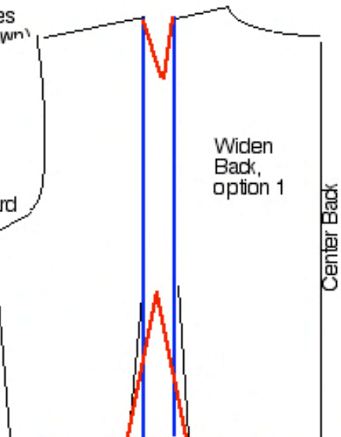
Blue lines are the lines you draw, then cut and move Red lines are new or altered darts
